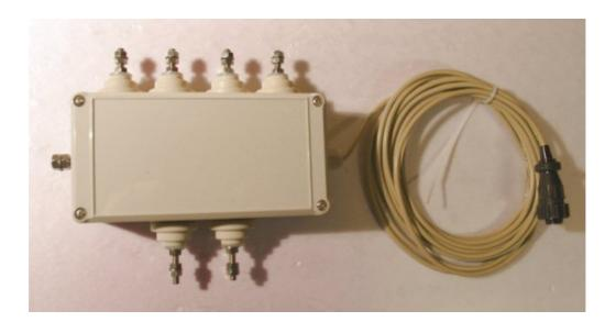
The remotely controlled Antenna Selection Unit (ASU-502) is designed for use with the hamware.de AT-502 tuner, but it can also be used as a stand-alone unit. It is designed to provide maximum isolation between the two sets of antenna terminals with minimum impedance variation.
